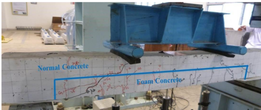
Figure 13. Composite beams with lightweight foamed concrete segment
