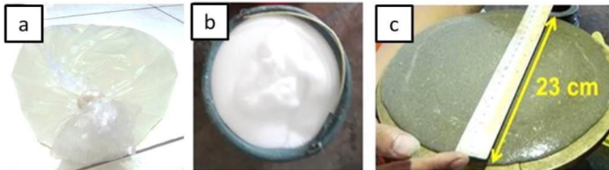
Figure 2. (a) Foam agent, (b) Foam, and (c) Foam concrete slurry
